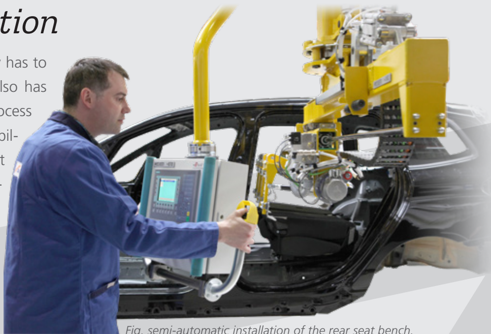
Fig. semi-automatic installation of the rear seat bench.
